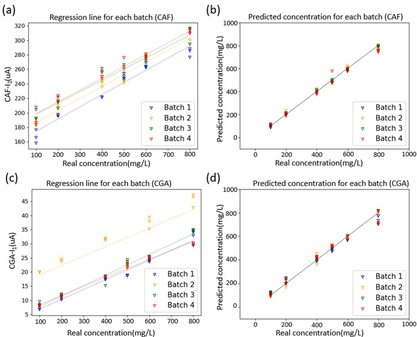
Fig. 7. (a) Linear regression lines for CAF measurements from different batches, (b) predicted results for CAF measurements from different batches using the ANN model, (c) linear regression lines for CGA measurements from different batches, (d) predicted results for CGA measurements from different batches using the ANN model.
