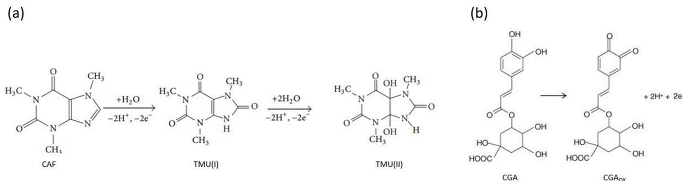
Fig. 2. Oxidation mechanisms of (a) caffeine and (b) chlorogenic acid.
