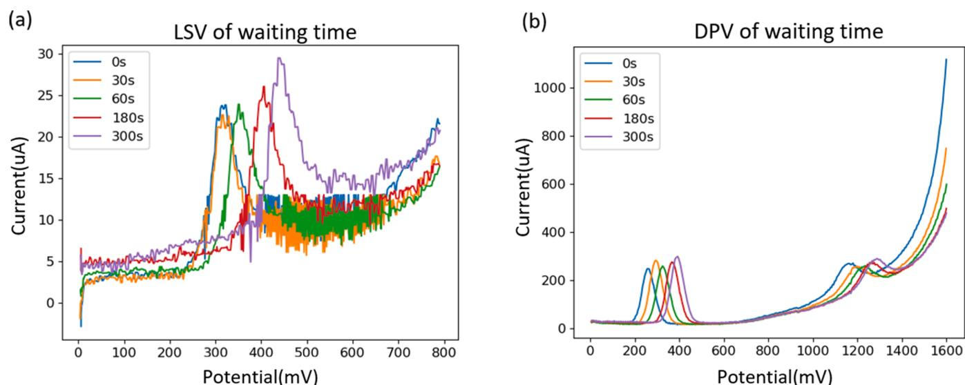
Fig. 8. (a) LSV measurement plots for samples with different waiting times of 0, 30, 60, 180, and 300 s. (b) DPV measurement plots for samples with different waiting times of 0, 30, 60, 180 and 300 s.
