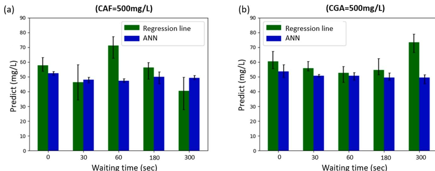
Fig. 9. Prediction results for (a)CAF measurements and (b) CGA measurements using the calibration line method and ANN model for waiting times of 0, 30, 60, 180, and 300 s.
