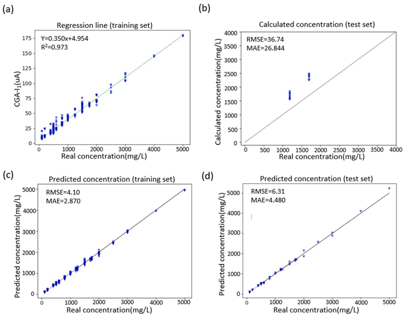
Fig. 5. (a) The linear regression line for the CGA training set, (b) calculated results using linear regression equation for the CGA test set, (c) predicted concentration using ANN model for the CGA training set, and (d) predicted results using ANN model for the CGA test set.
