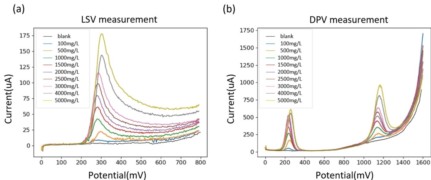
Fig. 3. (a) The plot of LSV measurement for different CGA concentrations (b) The plot represents the DPV measurements for different concentrations of CAF and CGA.
