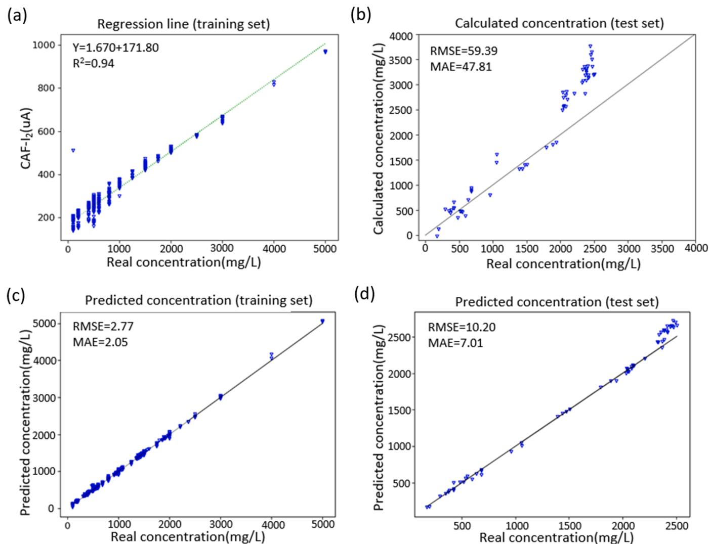
Fig. 4. (a) Linear regression line for CAF training set, (b) calculated results using linear regression equation for CAF test set, (c) predicted concentration using ANN model for CAF training set, and (d) predicted results using ANN model for CAF test set.
