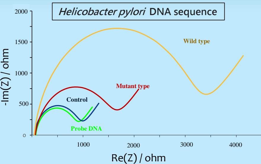
▲ Electrochemical Impedance Spectroscopy
